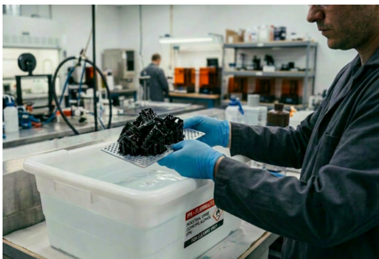
Additive Manufacturing Technician Cleaning Resin Parts Using IPA
