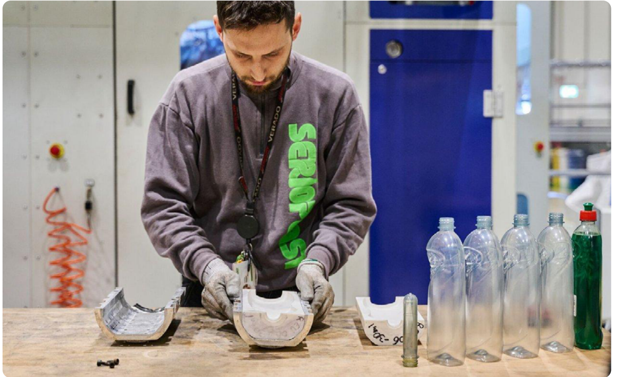
The mold 3D printed with Rigid 10K Resin is manually polished and then assembled into a metal frame.
