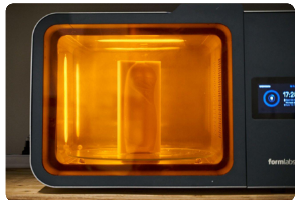
After washing, the supports are removed and the mold is post-cured.
