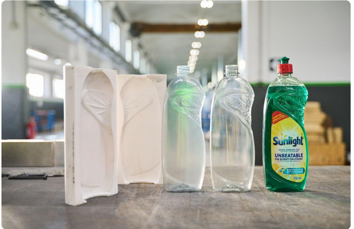
Bottles produced with a 3D printed tool are nearly indistinguishable from the final product produced through traditional metal tooling processes. From left to right: the two-part mold 3D printed with Rigid 10K Resin, a bottle produced with the mold 3D printed with Rigid 10K Resin, a bottle produced with a metal mold, and a labeled prototype bottle for customer testing.
