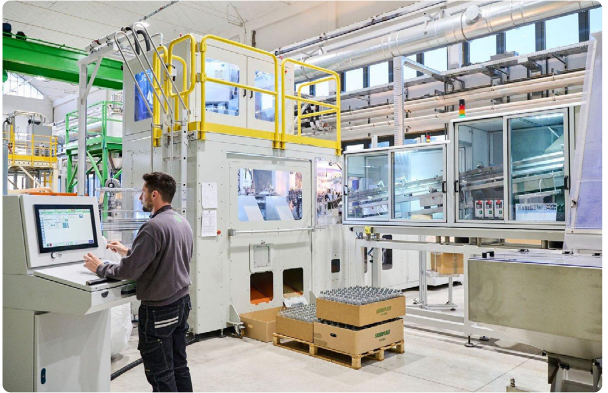
Seriomac UNIX 4 Cavities SBM machine from Serioplast in their R&D facility in Italy. Together with Unilever, they developed a new workflow for using 3D printed molds in this large-scale industrial manufacturing equipment.
