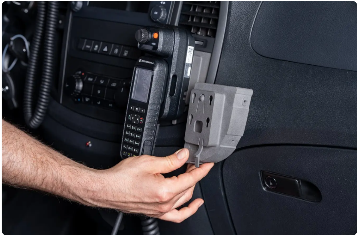
The radio mount is a great example of customization. The attachment to the console is the same for each Mercedes van, but the overall assembly can be easily modified with different mounts for radios of various manufacturers.
