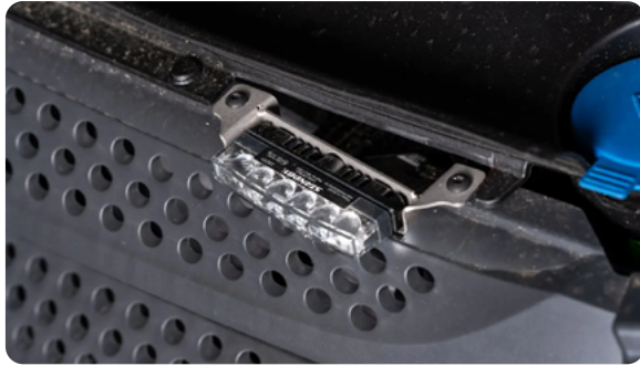
Custom mount for the LED front flash lights on police vans. The team traditionally used sheet metal forming to produce these parts.
