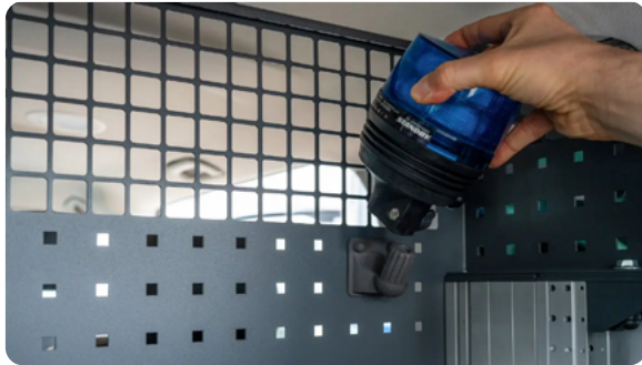
Clip-on mount in the cargo hold for a removable emergency light. Custom mount for the LED front flash lights on police vans.
