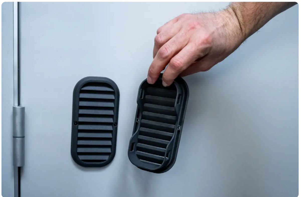
This air vent is a one-way valve that separates the black from the white compartment in a special vehicle for arson investigation. It's an assembly with a relatively complex design consisting of three components that are screwed together. The team initially tried to produce it with FDM 3D printing, but ran into challenges due to the circular shape and thin walls, and moved to SLS 3D printing as it offers more design freedom.
