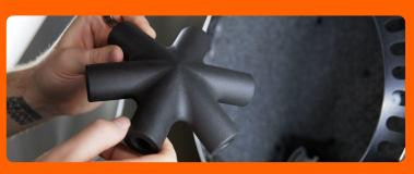
Fuse Blast Polishing System can create consumer-ready surface finishes even on organic shapes and in hard-to-reach areas, like on this connector part.
