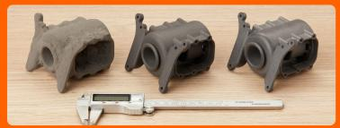
Left to Right: Pre-Fuse Blasted part with some unsintered powder in its negative features and less defined edges. Fuse Blast-cleaned part with no unsintered powder. Cleaned and polished part after using Fuse Blast Polishing System.
