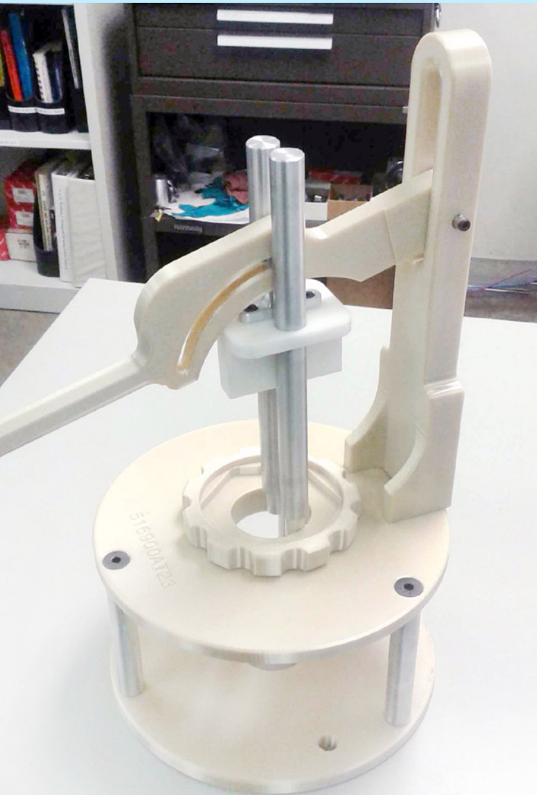
This pressing tool incorporates ULTEM™ 9085 resin material.
