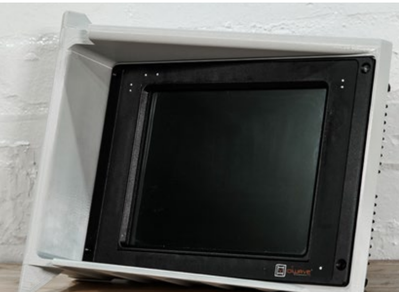
The lighter-colored bezel surrounding the video screen was 3D printed using Kimya PC-FR fire retardant material.
