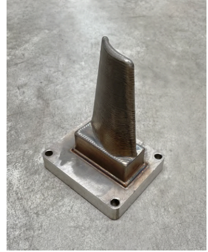
Figure 8. Turbine blade printed (DED) on the base
