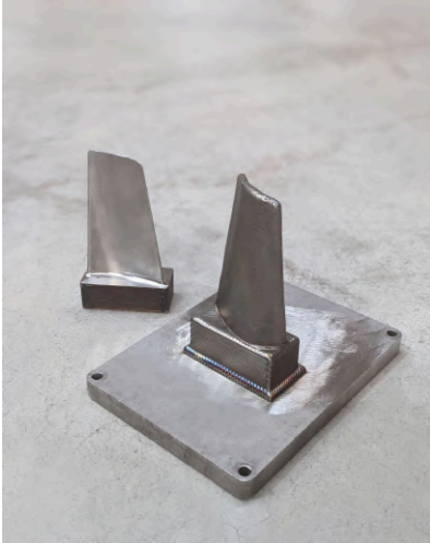
Figure 6. Comparison between turbine blade printed on the base and after removing and machining
