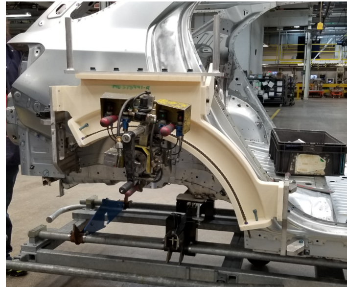
The wheel arch hemmer tool (ivory) made from ASA thermoplastic.
