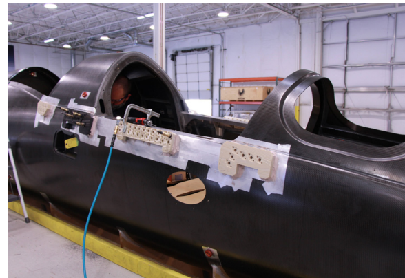
3D printed drill guides being used to drill fastener holes through a carbon fiber reinforced plastic (CFRP) and titanium stack-up in the XB-1 fuselage.
